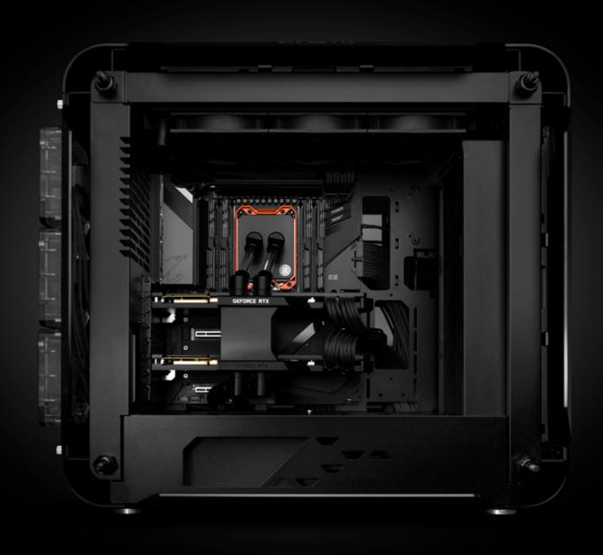
Derived from an obsession with liquid cooling this build reveals everything, an instant reminder to appreciate all things plexi and RGB. A Reflection distribution plate and EK-Loop vertical GPU bracket are used to translate all of the components into a single plane, maximising the intricate details and vibrant coolant that can be seen.
